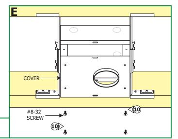
**10:** Loosen the four #8-32 screws on the front of the housing, to remove the cover.
