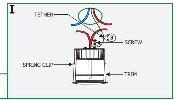
**3:** After installing drywall and finishing it, align the tether terminal to the trim tab and secure it by replacing the Phillips screw.
