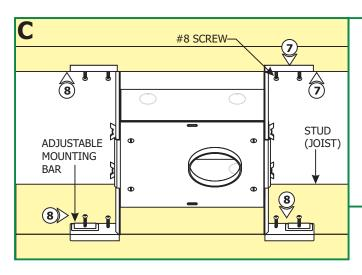
**NOTE:** The adjustable mounting bars mount to joists (studs) that are spaced 16" to 24" apart.
