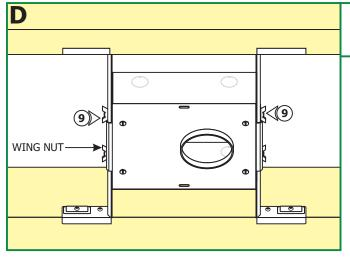
**9:** Slide the housing to desired position. If necessary loosen the wing nuts to ease the sliding. After the desired position is achieved tighten all the wing nuts.
