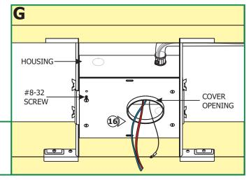
16: Feed the black & red output wires from the LED driver along with the tether through the cover hole. Mount the cover to the housing with the four #8-32 screws. The hole should be over the tether and the solid side will cover the LED driver.
