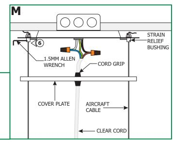
**5:** If the glass shade is not level horizontally, slide the cover plate down to expose the mounting plate.
