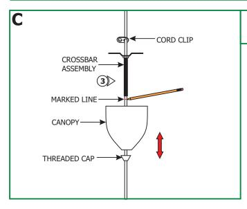
**3:** Adjust the fixture height by sliding the cord up or down through the crossbar. Make a line behind the crossbar assembly when desired height is determined.
