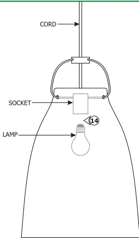
**CAUTION:** To reduce risk of a burn or electrical shock during lamping, disconnect the power to the fixture.
