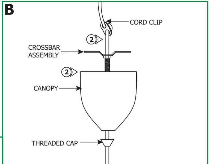
**2:** Loosen the threaded cap, to expose the crossbar assembly and also entangle the cord from the cord clip.
