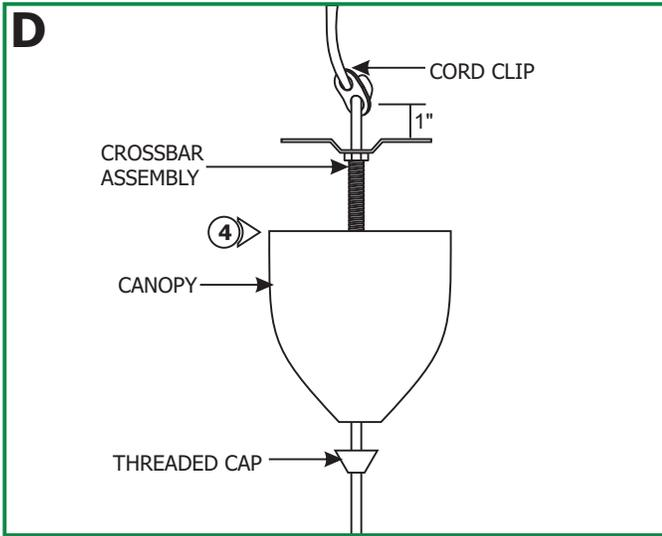
**4:** Place the cord clip 1" above the marked line by feeding the cord through the second hole on the cord clip and pulling it out to lock in place.
