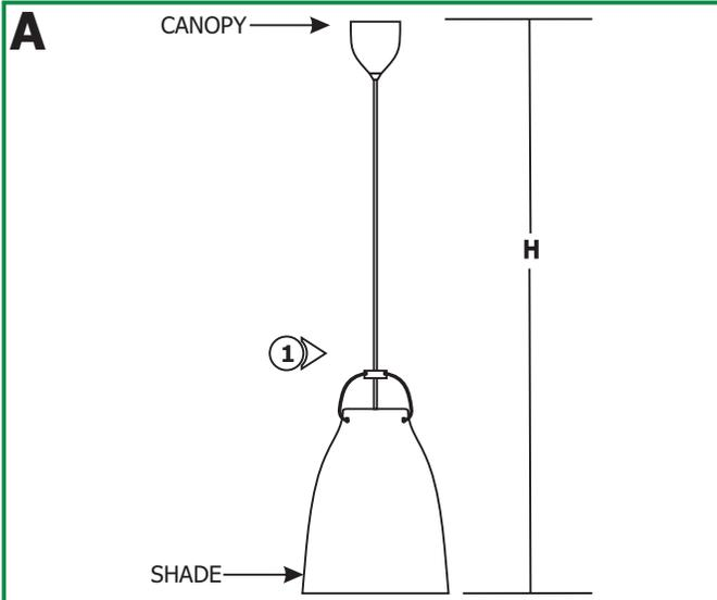
**1:** Determine the desired fixture height (**H**), from the bottom of the shade to the top of the canopy.
