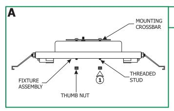
**1:** Remove the two thumb nuts from the threaded studs and detach the mounting crossbar from the fixture assembly.
