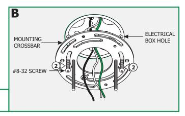
**2:** Mount the mounting crossbar to the electrical box holes with the two provided #8-32 screws
