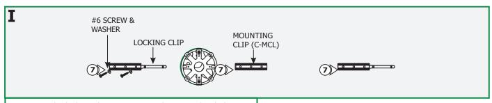
**7:** Line up the locking clips & mounting clips to anchor holes and secure them by tightening the two #6 screws with washers under the head into each clip.
