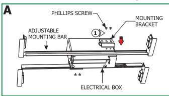
**1:** Mount each adjustable mounting bar to one side of the electrical box (mounts to any side of the housing depending on the orientation of the channel) and secure them with the mounting brackets and two Phillips screws provided.
