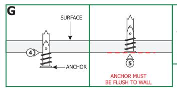
**NOTE:** Steps 4 and 5 are for drywall mounting. Omit these steps if mounting the clips to a wood surface directly.
