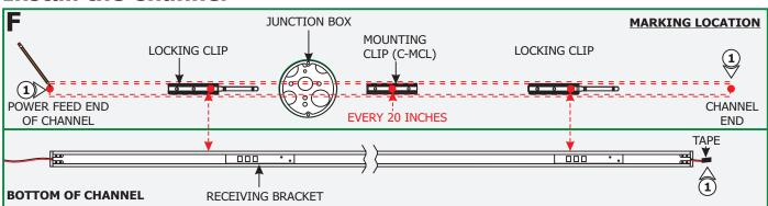
**NOTE:** Remote power supply must be installed within 40ft of electrical box. The low voltage 24V DC wires must be present in electrical box before installing the channel. Refer to the installation instructions provided with the power supply.
