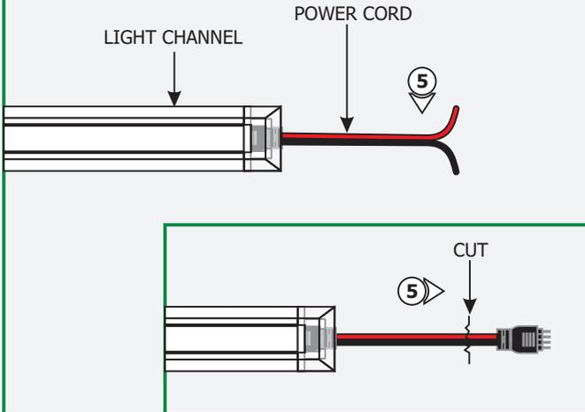
**5:** Cut the other end of the power cord (male or female) and discard it. Strip the wire end for connecting it to the power supply.
