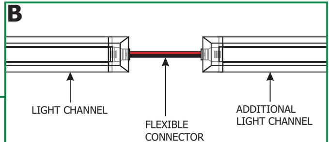
**NOTE:** Multiple light channels up to total of 25 feet long can be connected together with the flexible connectors. Refer to the instructions provided with the flexible connectors.
