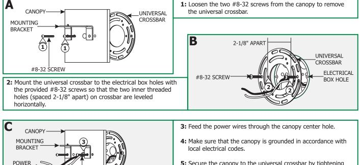
**5:** Secure the canopy to the universal crossbar by tightening the two #8-32 screws through the mounting bracket holes into the two inner threaded crossbar holes.
