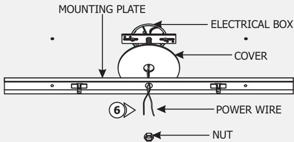
**7:** Slide the cover and mounting plate center hole onto the crossbar threaded nipple and secure it with the nut provided.
