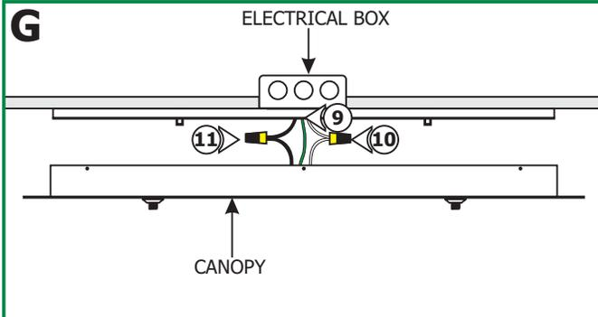
**9:** Make sure the mounting plate is grounded in accordance with local electrical codes.
