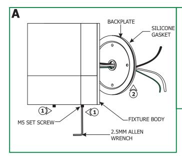
**NOTE:** Use the universal crossbar (provided) when mounting the fixture to an octagon box. There will be a 1/16" gap between the fixture and the wall when the universal crossbar is used. Caulking around the fixture will be needed when the universal crossbar is used in outdoor applications.
