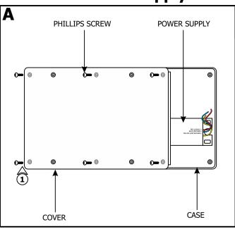
**1:** Loosen and remove the six Phillips screws on the front of the power supply cover to remove the cover from the case.
