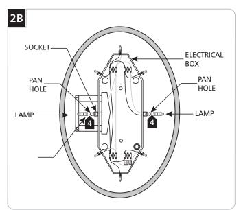
4 Handle the lamp with a soft cloth to prevent the natural oils on the fingertips from collecting on the lamp. Pull the lamps out. This will clear the two side pan holes for installation.
