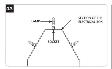
Use **MAX 40** Watt type T4, G9 base bi-pin halogen lamp in each socket.
