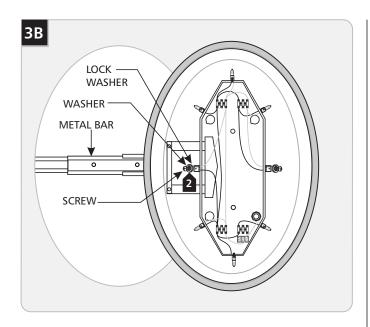
2 Mount the pan to the metal bar with provided washers, lock washers and the screws.
