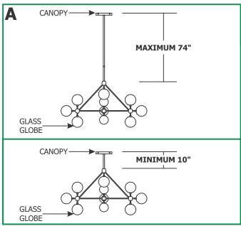
**NOTE:** Determine the desired overall fixture height using the 8" stem only or using additional combination of 20" and 12" stems for a maximum overall extension of 74".
