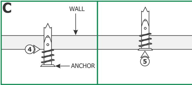
**4:** Tap the anchors onto the marked points up to the threaded portion with a hammer.
