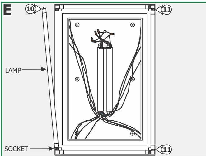
**CAUTION:** To reduce risk of a burn or electrical shock during lamping, disconnect the power to the fixture.
