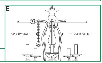
**7:** Install the six pieces of crystal marked "A" into each hoop at the top end of the curved stems.
