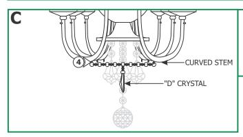
**4:** Install the six pieces of crystal marked "D" into the hoops located on the bottom of each curved socket stem, so that one end is hooked into one socket stem hoop and the other end into the adjacent socket stem hoop. Each curved socket stem will hold two crystal key rings when all crystals are installed.
