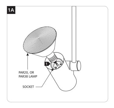
**NOTE:** Turn off power to the system before installing, removing, or relamping the fixture.
