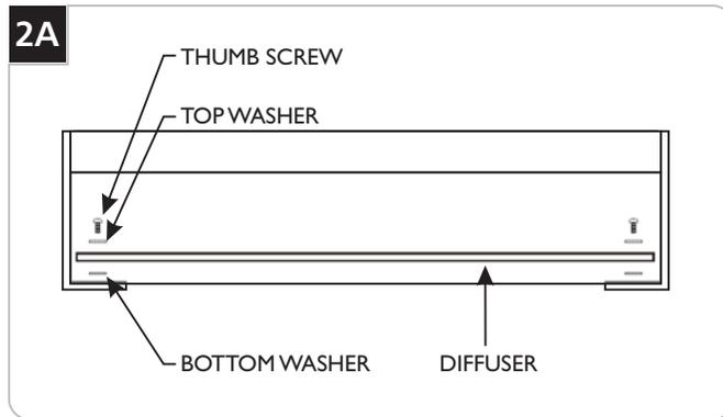
**CAUTION:** Do not over tighten the diffuser screws. Over-tightening may break the glass and result in injury. Ensure that all the washers are properly in place.
