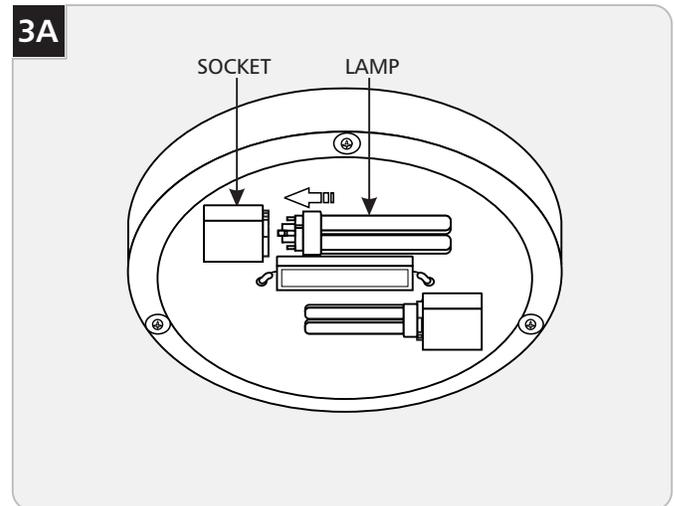
**CAUTION:** To reduce the risk of a burn or electric shock during lamping and re-lamping, disconnect the power to the fixture.
