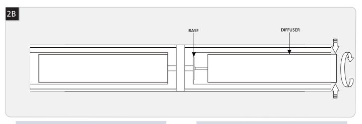
CAUTION: When installing the diffuser, apply even pressure on each side of the diffuser by using both hands to screw it in place. DO NOT OVER TIGHTEN the diffuser. This may break the glass resulting in injury.
