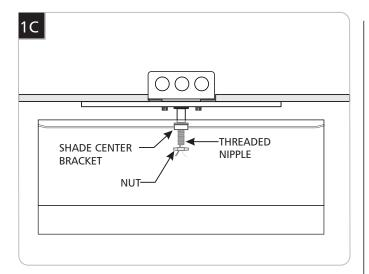
5 Insert the shade onto the threaded nipple through the shade center bracket. While holding the shade in place, screw in a nut and secure the shade by completely tightening the nut.
