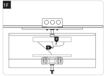
8 Connect the fixture white wire to the neutral power line wire with a wire nut.
