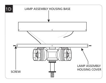
6 Detach the lamp assembly cover from the base by loosening and removing the four screws.
