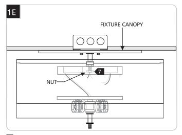
**7** Install the housing base to the threaded nipple and secure it by screwing on a nut and completely tightening it .
